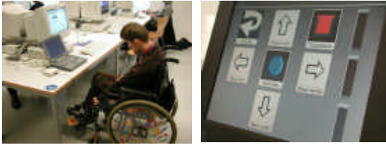
Input via single foot switch, autom. Scanning, scan time 0.8 sec, appr. 3,600 icons (symbols) structured in appr. 115 menus (levels). Used for writing Source Code as to be done in the framework of informatics courses, personal report by student (in German) to be found on http://www.fortec.tuwien.ac.at/seminar
