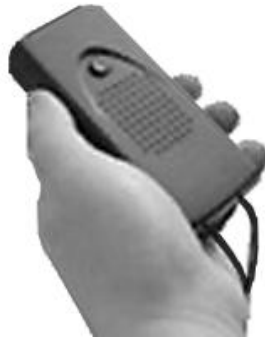
Abb. C 1.24: Empfänger des "Talking Signs" Systems.
