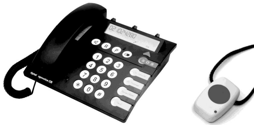
Abb. C 4.23: Notruftelefon: links Zentraleinheit; rechts: Handsender (Tiptel Ergovoice CR).
