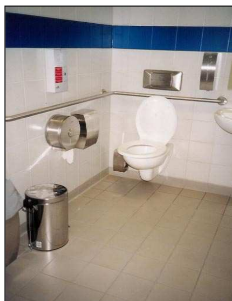
Fig. 14-7 and Fig. 14-8: UA at Athens’ International Airport: tactile orientation marking at the departures hall and a family-size (PwD’s) toilet (not properly equipped!)
