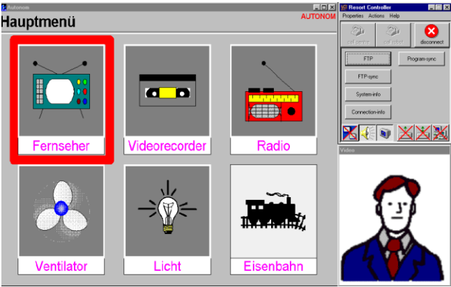
Fig. 3: Prototype of a more complex ECS user interface. On the left hand side the screen displays the RT system, in this case a Technical Assistive System for motor and multiple impaired persons called “Autonomy”. In the upper right hand corner the Resort Controller, in the lower right hand corner the video channel.
