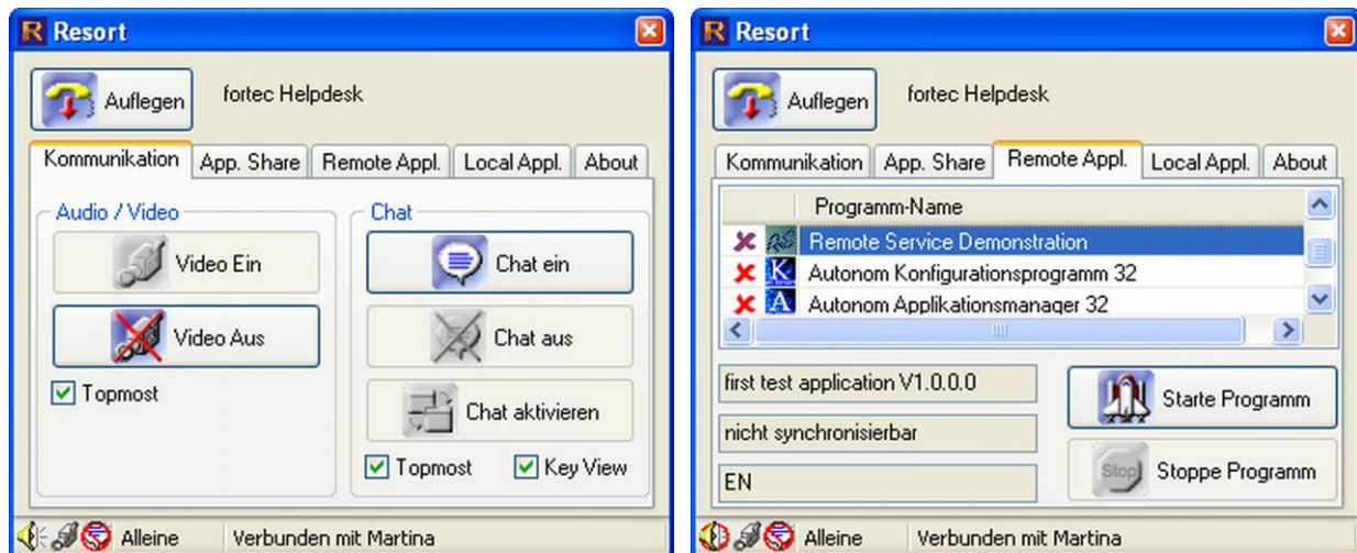
Figure 4. Screen Shots from RESORT Service Centre during a Tele-Service Session. Left picture shows controls for video and text communication, right picture contains controls for remotely starting and terminating RT applications at the client side
