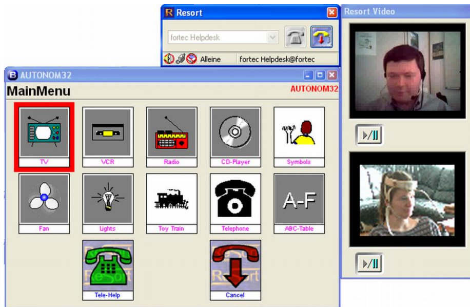
Figure 3. Screen Shot from a RESORT Client during a Tele-Service session in Vienna. A non-speaking head stick using person runs an environmental control and communication system called AUTONOMY [15], [17] which is equipped with a RESORT Interface. The service centre can be called from inside the AUTONOMY system
