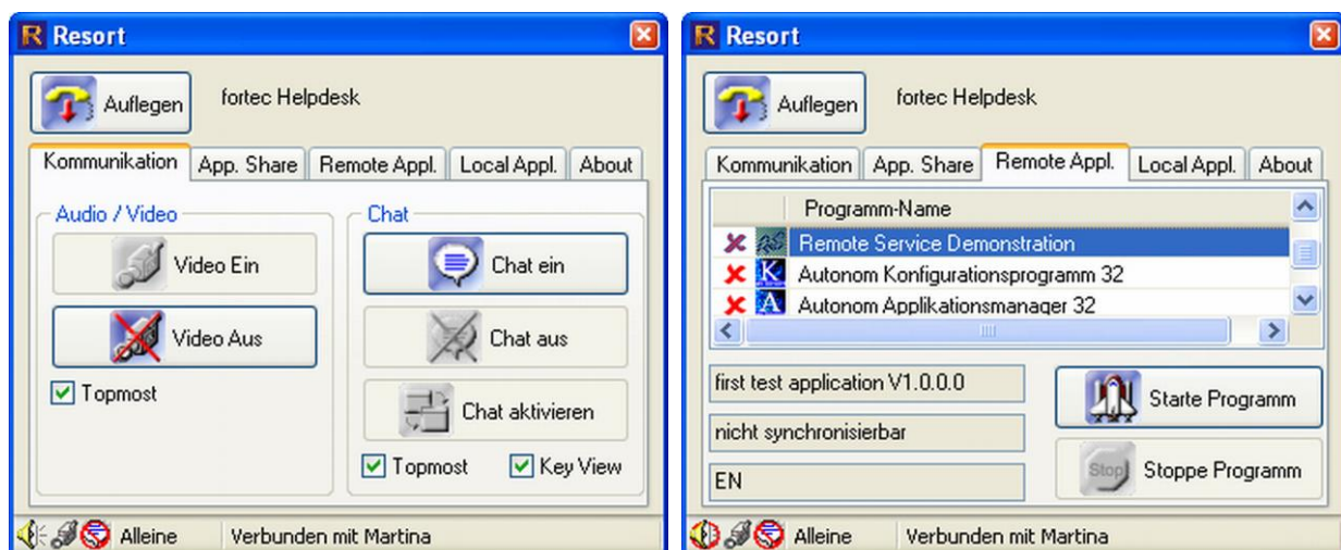
Figure 4. Screen Shots from RESORT Service Center during a Tele-Service Session. Left picture shows controls for video and text communication, right picture is showing controls for remotely starting and terminating RT applications at the client side (Prototype version written in Delphi running on WindowsXP)
